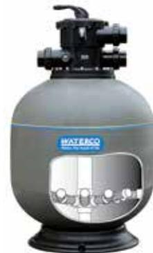
*The Micron ECO features an internal hydraulically-efficient system, which is designed to facilitate energy and water savings. Its unique 'fish tail' laterals ensure better water flow distribution through the filter's media bed, enhancing its filtration and backwashing efficiency.*
