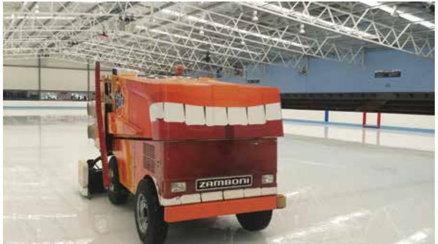
*Zamboni ice re-surfacer machine shaving off the top layer of ice.*
