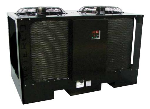
Electroheat PRO 96kW heat pump commercial grade pool heater features electronically controlled temperature management, fault diagnostic system and inbuilt protection devices and operates with dual high performance hermetic scroll compressors using R410A refrigerant for increased efficiency.
