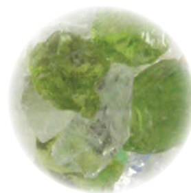
Grade 3 3.0 - 6.0mm (equivalent to Pea Gravel)
