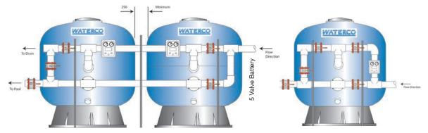
Double Filter 5 Valve Battery
