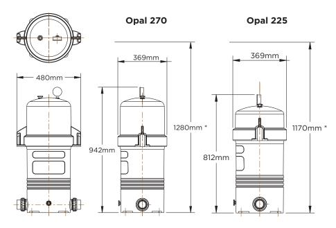
\* Minimum Clearance Height to Remove Cartridge
