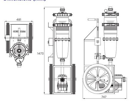
Note: Standard Ultravac comes with a 0.5Hp Supastream pump and Multicyclone Plus MC12 (40ft² cartridge). Other combinations available upon request. Vacuum hose is not supplied.
