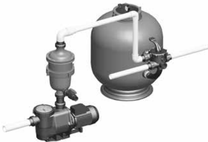
Typical Installation with a Sand Filter
