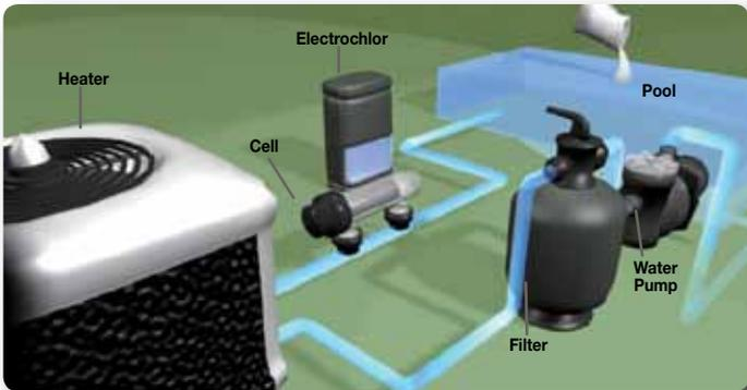
The Electrochlor is plumbed directly in-line with the pool equipment, typically after the heater
