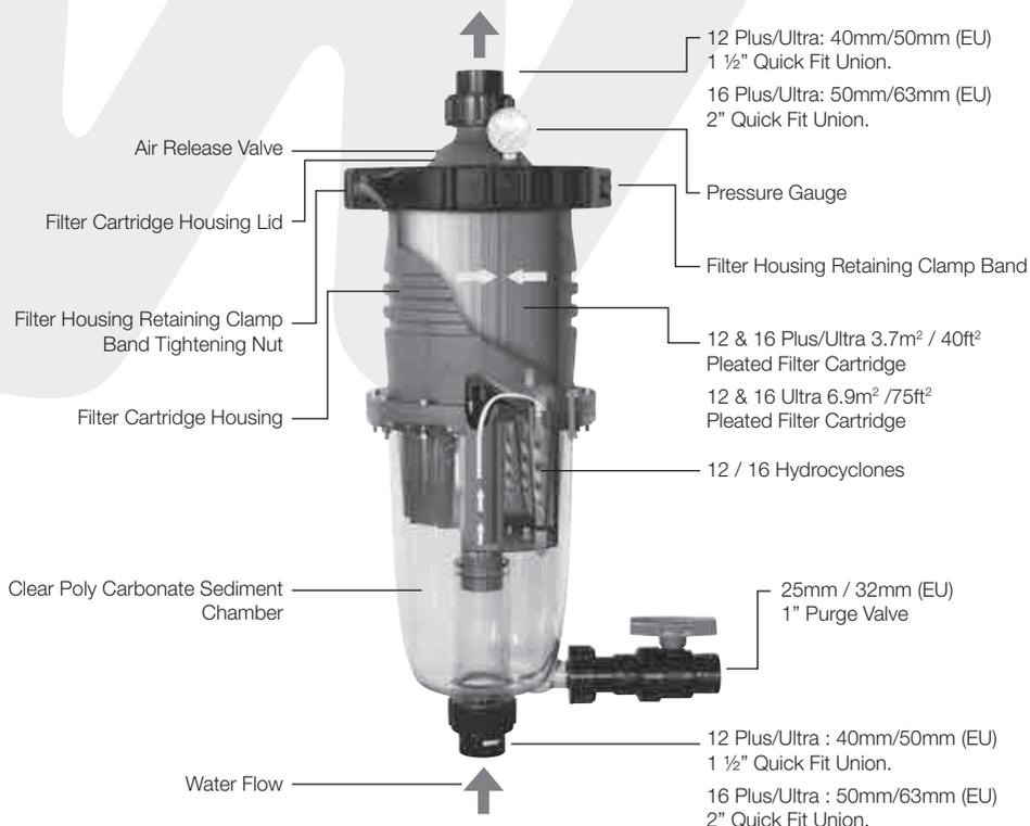
**Note:** The MultiCyclone Plus/Ultra centrifugal section is designed to filter sediment that is heavier than water; floating debris cannot be filtered out by centrifugal filtration.
